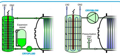
The left heat exchanger configuration with the **CRYOFLUID** is used for liquid heat transfer fluids such as typically silicon oil or 3M segregated hydrofluoroethers (HFEs), while the **CRYOBLOW** configuration on the right is intended for use with gaseous heat transfer fluids (pressurized  $GN_2$  or helium).
