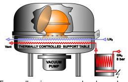
For smaller size vacuum chambers where only a temperature controlled table is required, cast aluminium heat exchangers (see HEXAL brochure) can be offered as alternative. Only liquid and hot gaseous nitrogen are used resulting in dramatically reduced overall consumption.
