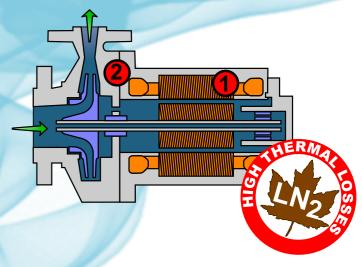
The same remarks are valid for the encapsulated motor version where the fluid is heated by the eddy currents between rotor and stator 3.
