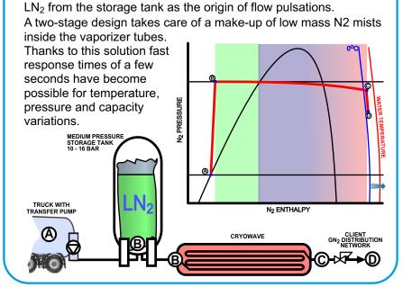
**CRYOWAVE** by RLD is a modular design using tubes optimized
