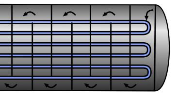
**CRYOWAVE** by RLD is a modular design using tubes optimized with tube inserts for an uniform and improved heat exchange over the total tube length. Moreover, RLD has identified the sub-cooled  $LN_2$  from the storage tank as the origin of flow pulsations.
