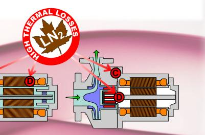
All energy (mechanical or thermal) transmitted to the liquid must be compensated by an equal amount of refrigeration in order to maintain a stable cooling temperature.
