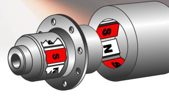
Inner magnets, non-magnetic bell and exterior magnets of a magnetic coupling set
