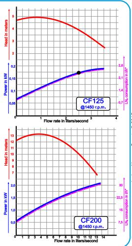
\*LN<sub>z</sub> consumption in 4 graphs is in *l*/h, • LN<sub>z</sub> storage pressure: 2 barg • density of heat transfer liquid: 1 • working temperature: -50°C
