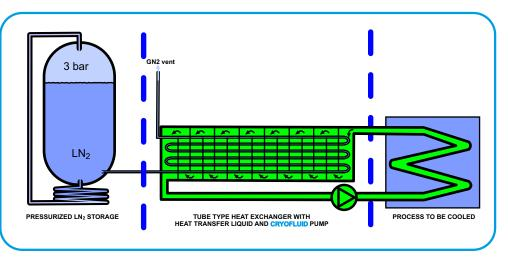
As opposed to commonly available designs (without modification or customization,) the **CRYOFLUID** concept is fully tailor-made and governed by the objective to reduce the total energy absorbed by the cryogenic fluid through the pumping process.
