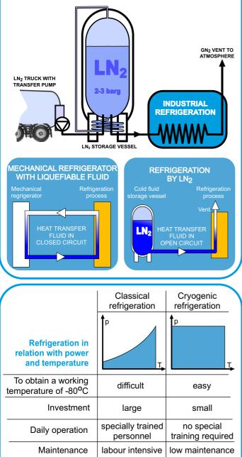
When used in continuous operation LN<sub>2</sub> becomes competitive for temperatures lower than -50°C. For batch operation LN<sub>2</sub> can be competitive up to -20°C specially when large refrigeration power is required.
