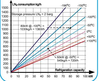
RLD amongst other companies, has made it their goal to reduce  $LN_2$  consumption in thermal processes. They have invested in development of new cryogenic components, thus dramatically economizing liquid nitrogen during the lifetime of installations using cryogenics.
